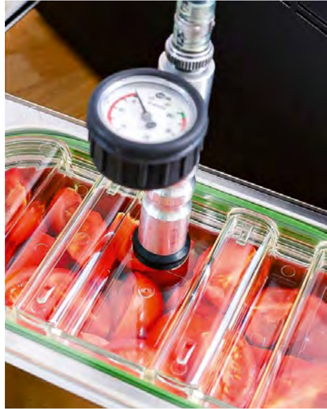
Vacuum containers can be placed under vacuum in connection with a Komet machine.
